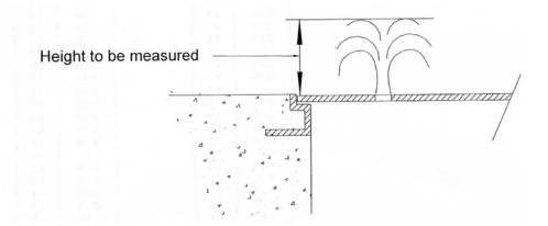
Example: Measured height of plume exiting pick/vent hole is 1 inch from a  $\frac{1}{2}$ -inch vent hole and there are 4 vent holes. The total volume per minute would be .94 gpm per hole (from attached chart) or 3.76 gpm total (.94 gpm x 4 holes) from the manhole cover. If the SSO lasted one hour, the total wastewater lost would be 226 gallons (3.76 x 60 = 225.6).
