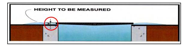
Example: The measured height of the plume exiting the ring of a 36-inch manhole is 1 inch. The total volume per minute would be 13 gpm from around the ring of a 36-inch manhole cover (from the attached chart). (Calculate the amount exiting the pick hole(s) and add to the total being lost around the ring). If the SSO lasted one hour the total wastewater lost would be 780 gallons ( $13 \ge 60 = 780$ ).
