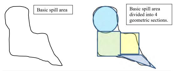
Determine the area of each of the geometric sections adding them all together to determine the total area of the spill.
