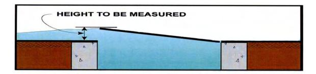
Example: The measured height of the plume exiting the side ring of a 24-inch manhole is 2 inches. Based upon the data provided in the Area Calculation Chart below, a 2-inch plume from one side of a 24-inch manhole cover provides 0.524 square feet of area. The velocity of the flow is estimated at 4 ft/sec (visual observation) with the assumed duration of the flow lasting for one hour. The total amount of the SSO is estimated at 56,441 gallons (.524 x 4 x 60 x 7.48 = 56,441)
