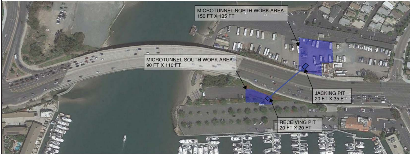
PCH Crossing Work Areas
