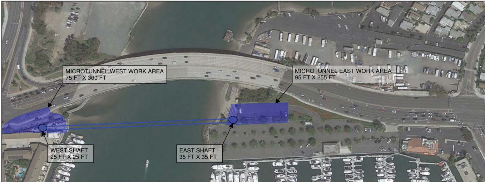
Newport Bay Channel Crossing Work Areas
